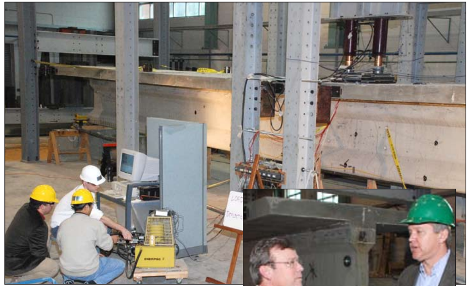
USC Engineers monitor the 12-inch bend in the 59-foot concrete girder after 221,000 pounds of pressure is applied.
