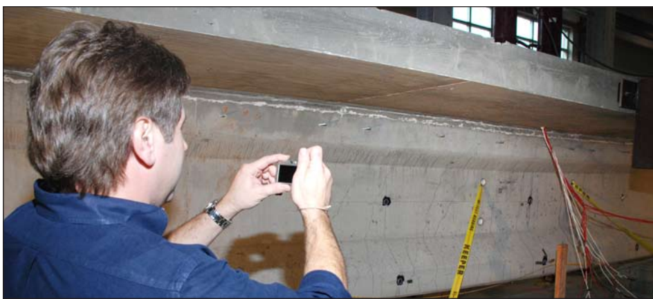
Merrill Zwanka photographs the cracks in the girder. Steel reinforcement rebar through the bottom of the girder also add strength to the structure.
