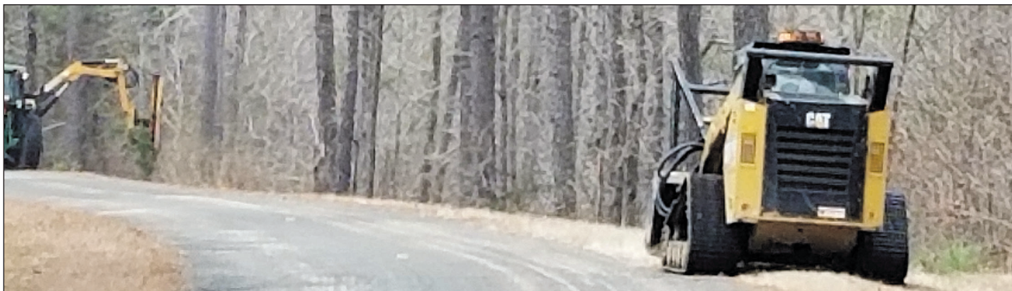
A skid steer with a forestry head waits as a buzz bar cuts limbs in the distance.
