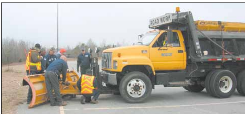
Union Maintenance employees attach a snow plow to a truck.
