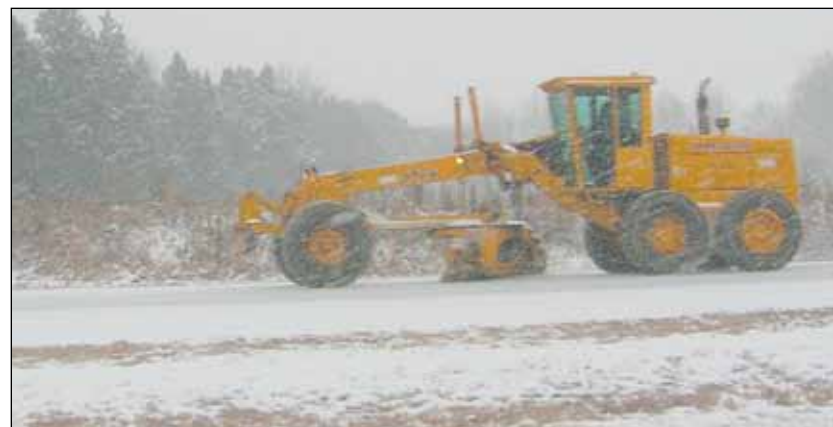
Harry Williams of Chester Maintenance uses a motorgrader to remove snow from S.C. 9.
