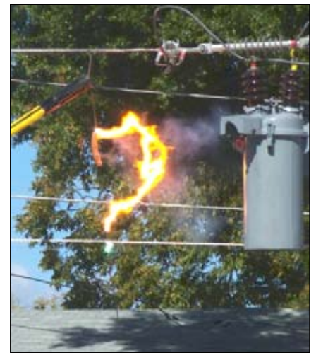
A hot dog, simulating a finger, bursts into flames when it touches a high voltage line.
