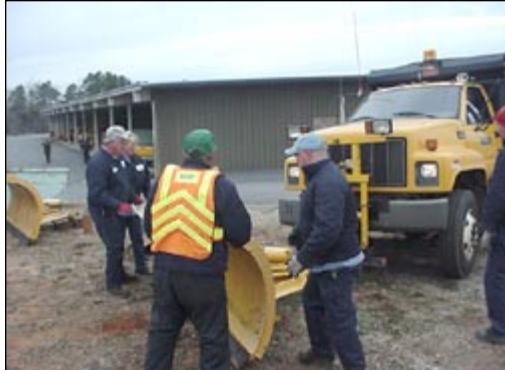
Crew members place scrapers on the dumptrucks.
